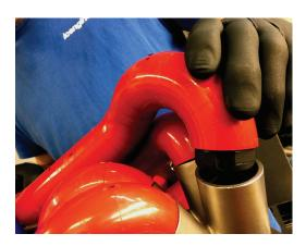
Any icengineworks<sup>®</sup> NPSeries modeling block can be anchored to an open pipe end of the manifold flange (starter pipe w/ round profile) or the turbocharger collector, to get the design started. Choose the design direction: following the gas flow direction (head to turbo), or going upstream (turbo to head) based on clearance, appearance, design complexity, welding sequence, etc.
