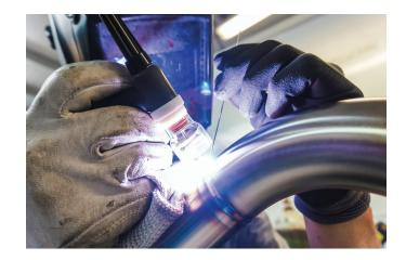
With all the curved and straight pipe sections cut per your Control Sheet, begin replacing them in your model. **Plan ahead the welding sequence to avoid dead ends.** Place at least 3 tacks around each joint that form the manifold runners for safety. Adjust accordingly until assembly is ready to be fully welded. Follow industry standard manifold welding procedures and techniques to complete your design.
