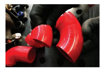
For the 1250NPSeries this requires the following blocks: For Short Radius elbows (SR, marked as 1-1/4"-CLR), use blocks labeled 45-deg/1" long **only** to form 1"-long or longer sections in 1" increments. For Long Radius elbows (LR, marked as 1-7/8"-CLR), use the 30-degree/1" long blocks **only** to form 1"-long or longer sections in 1" increments.
