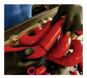
After setting up the first block in each runner using the neoprene block adapters, begin laying out your design. Connect 45-deg/90deg SR and LR block sections (single or multiples) with straight blocks to create manifold runners. Be sure to respect their intended compounded angle so the standard elbows can be used just as they come. Keep track of number of changes in geometrical planes of bend to control number of welds required as you build.
