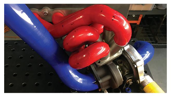
Thank you for choosing the icengineworks<sup>®</sup> NPSeries for precisely designing and fabricating turbo manifolds when using weld elbows in Sch5, Sch10 or Sch40. This manual covers pipe sizes 1-1/4"NPS (1250NPSeries) and 1-1/2" NPS (1500NPSeries).
