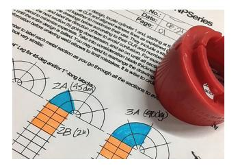
The process starts by coloring the pie sections in the drawings corresponding to each block section in the model. Properly label each section in the drawing identifying what cylinder it belongs to and its order in it to avoid confusion. For example: section 2C, meaning the third section in the flow direction in runner for cylinder 2. Straight sections will have their own label.
