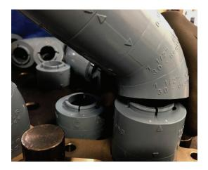
After setting up the first block in each runner in your design using the neoprene block adapters, begin laying out blocks to start the design. In ADVANCED DESIGN MODE you can use standard elbow angles and also create new combinations as explained previously to generate more sophisticated layouts.
