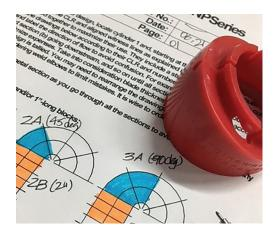
The process starts by designating pie sections in the drawings that correspond to each block section in the model. Properly label each section in the drawing identifying what cylinder it belongs to and its order in it to avoid confusion. For example: section 2C, meaning the third section in the flow direction in runner for cylinder 2. Straight sections will have their own label.
