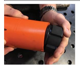
To get started, an intial icengineworks<sup>®</sup> plastic modeling block of your choice needs to be anchored to the open end tube coming from the exhaust header collectors, downpipe, catalytic converter, etc.
