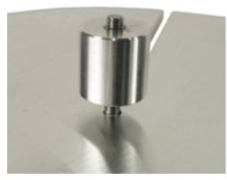
Install the 3/8"-16 flat head bolt through the back of the cutting plate to the front side and catch it by threading it into the supplied cylindrical aluminum stud. The aluminum stud is symmetrical so either end works.
