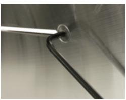
Using a 7/32" Allen wrench or ratchet, slowly tighten the bolt from underneath. Do this by holding the stud with your hand only while turning the bolt with the other.
